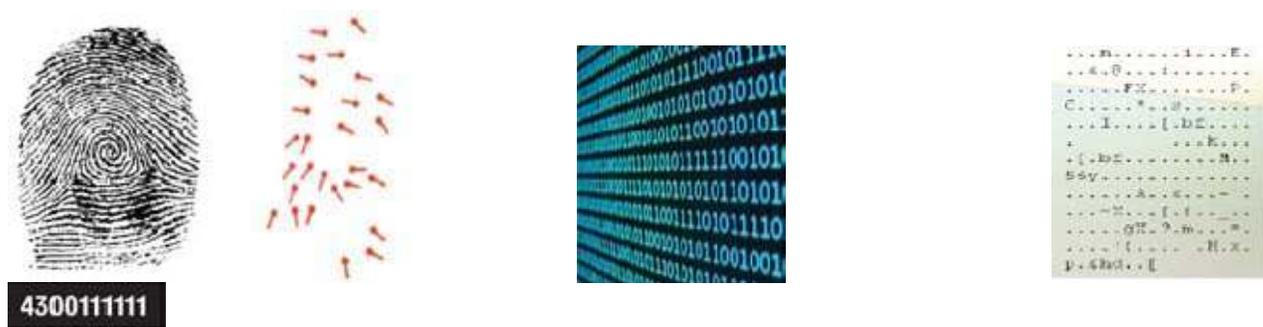
Finger is scanned. Unique points are identified. Points are transferred to binary number. Number is encrypted and identified. The fingerprint is destroyed! and equals the student's ID number.
